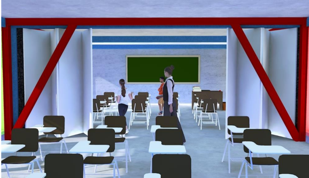
Figure 4- Interior view of retrofitted building. From [8]
